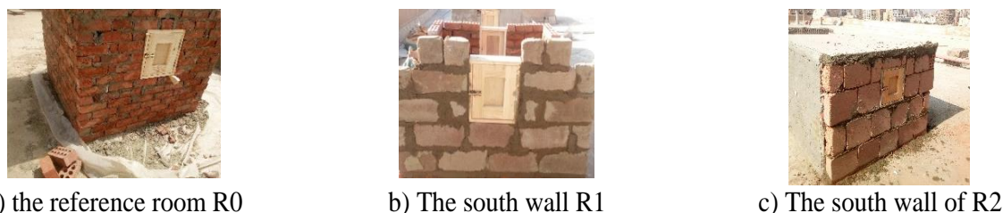
Fig.3. The experimental room models (R0, R1, and R2)
