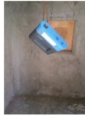
b) The inner temperature measuring device (OPUS10)
