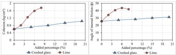
Figure 16. The comparison between the effect of adding crushed glass wastes and lime separately on soil's shear parameters
