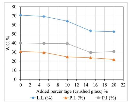
Figure 2. Graph of Atterberg limits against the percentage of crushed glass wastes
