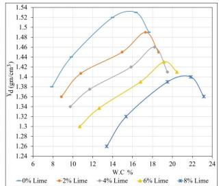
Figure 5. Compaction tests curves of the expansive soil-lime mixtures
