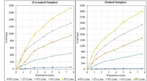
Figure 15. The penetration-load curves of the expansive soil-lime mixtures based on un-soaked/ soaked CBR tests
