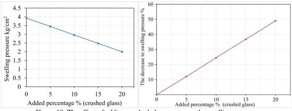
Figure 10. The effect of adding crushed glass wastes on the swelling pressure
