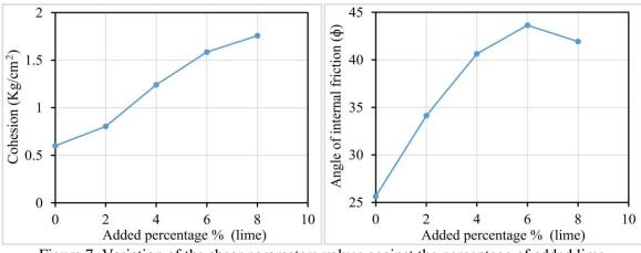
Figure 7. Variation of the shear parameters values against the percentage of added lime
