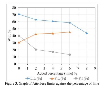
As clarified in Figure 3, by adding lime to the expansive soil, the liquid limit decreased from 70.75% to 43.65%, but the plastic limit increased slightly. The decrease in the liquid limit was much greater than the increase in plastic limit, which led to a decrease in the
