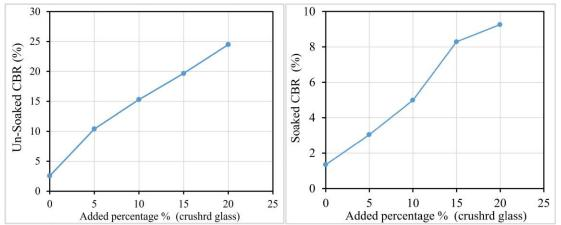
Figure 12. Graph of un-soaked/soaked CBR against added percentages of crushed glass wastes
