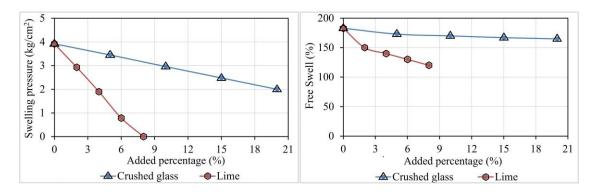
Figure 17. The comparison between the effect of adding crushed glass wastes and lime separately on soil's swelling properties
