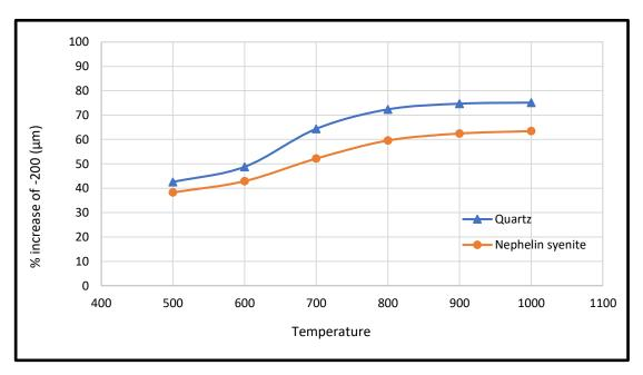
Fig. 2: Effect of heating temperature for 60 min. and water quenching on the percentage of increase of -200  $\mu m$  in the product
