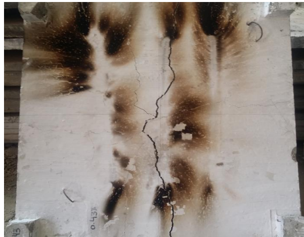
Fig. 10. Crack pattern of SFG11
