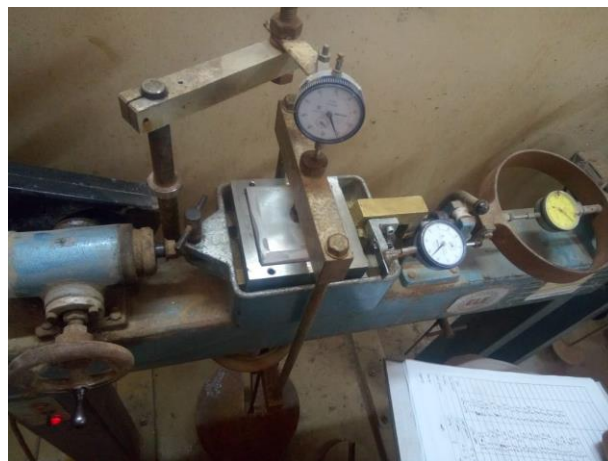
Figure 6 Direct Shear Box Device used in the research
