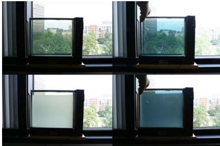
Figure 8. Demonstrates Glass Electrochromic Material (Telhan,2010)
