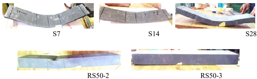
Figure 10: Deformations for Steel Beams
