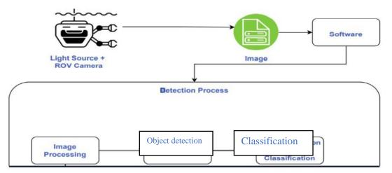
Fig.1: Diagrammatic representation of the integrated algorithm for ROVs using computer vision for underwater object detection and classification.
