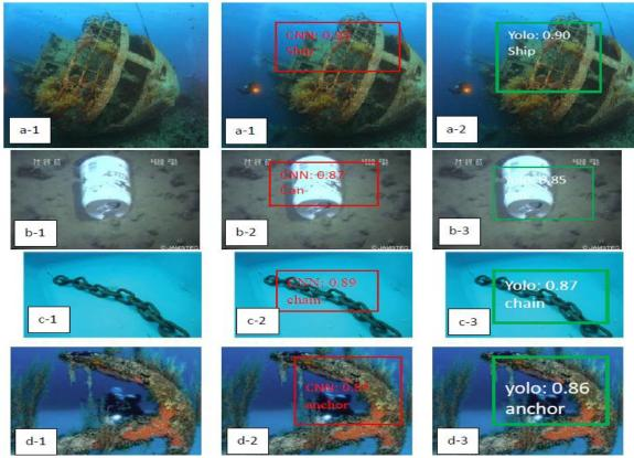
Fig.7: Object Detection and Classification Results Comparison a. ship b. can. c. chain. d. anchor
