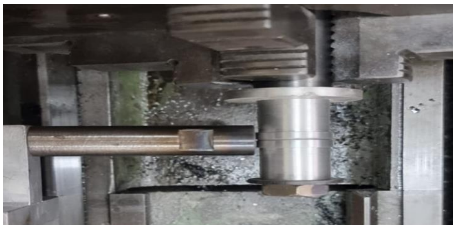
Figure 8: live view of flat tool with sample on the lathe
