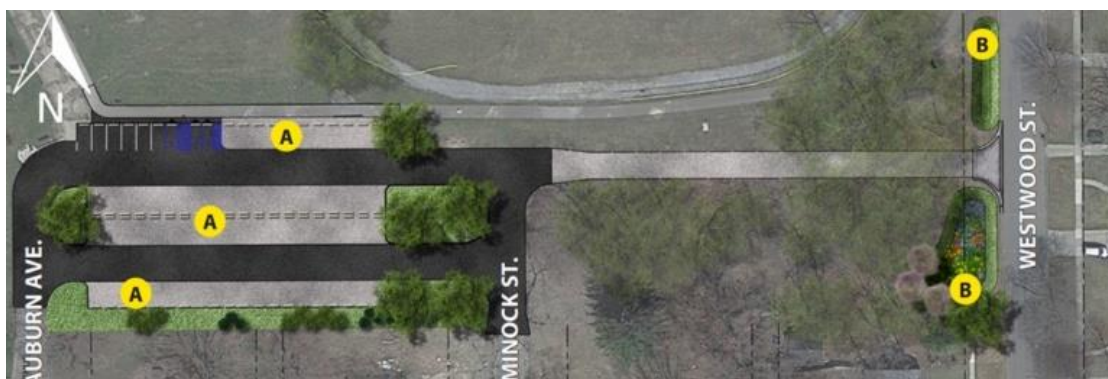
Fig.27: Proposed locations of new pervious stone parking spaces (A) and bioretention areas (B) at Stoepel Park No. 1 [44]
