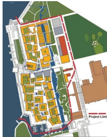
Fig.18: This plan of Bo01 diagrams the stormwater flow direction, the saltwater canal, and the smaller channels and basins that receive stormwater. Note the small aqua points in the interior of the project [31]
