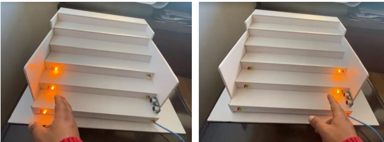
Fig. 17: On the right, yellow LED lights illuminated when sensor waves were interrupted for less than 2 seconds. On the left, yellow LED lights activated under the same condition.
