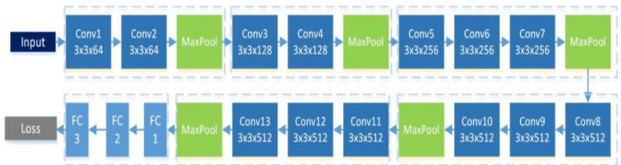
Fig. 3: Customized VGG16 Architecture.
