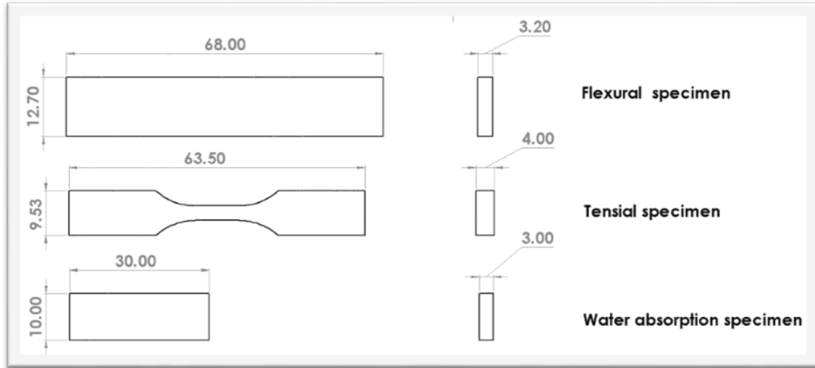
Figure 3. Geometry of tested specimens
