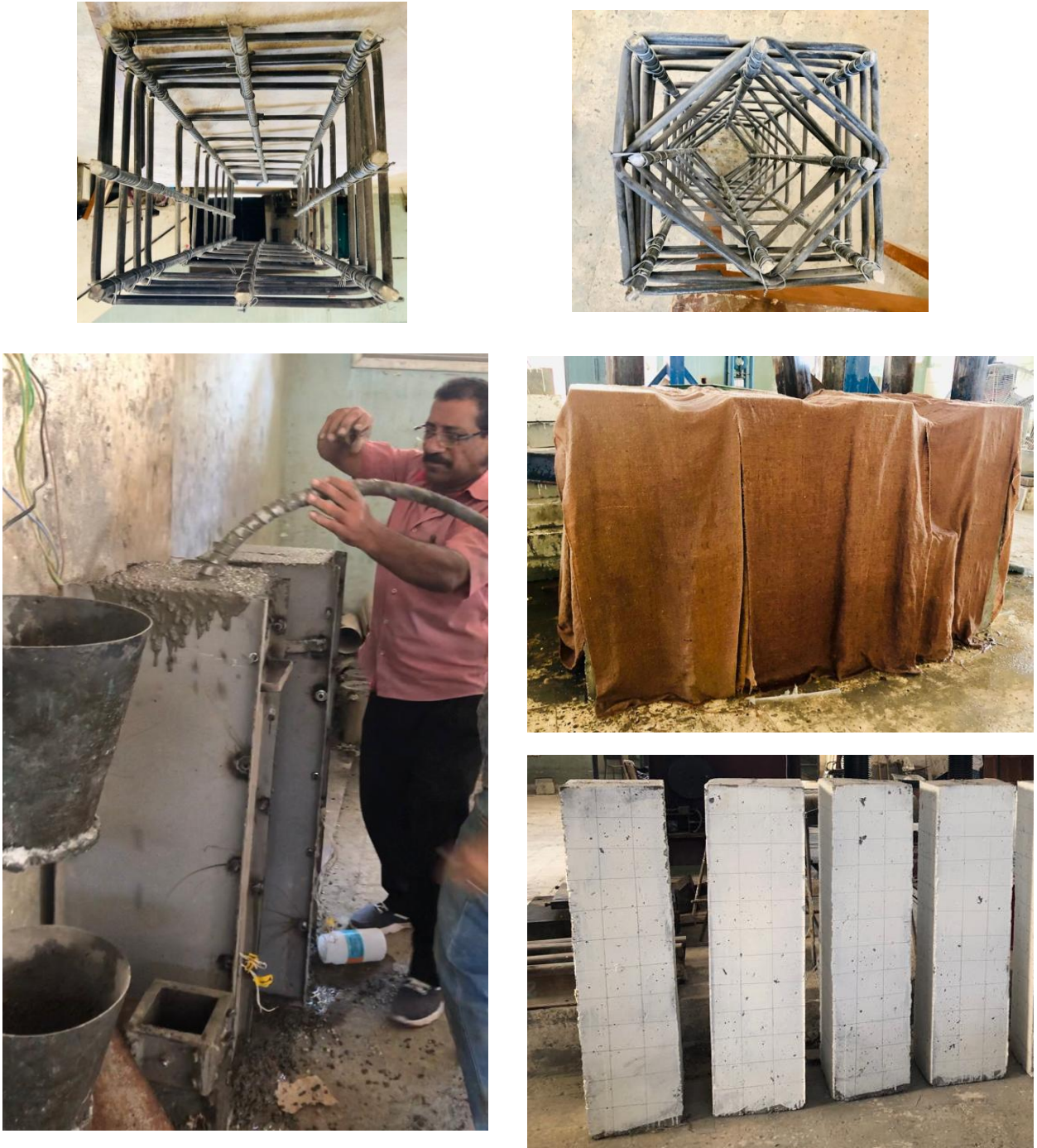
Fig. 4: cross-section of the columns with reinforcement details, concrete casting, curing process, and the columns are ready for testing.
