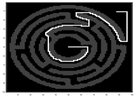
Fig.17. The path of a circular maze using 4_sector wave front method
