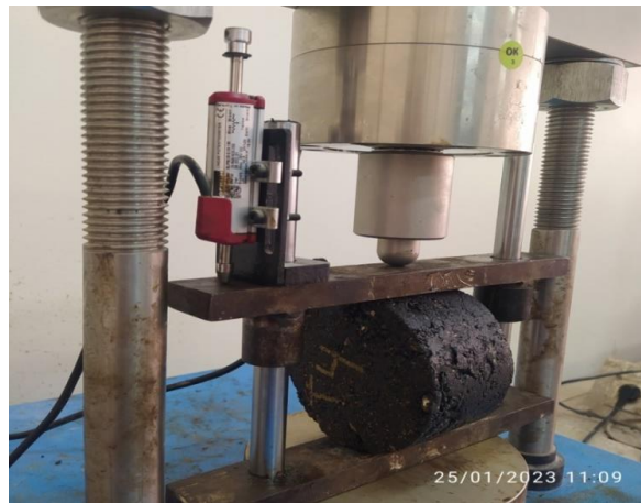
Figure 2: Indirect Tensile Strength (ITS) Test Setup
