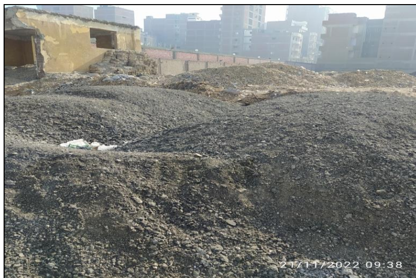
Figure 1: Stockpile of Unprocessed RAP Milling
