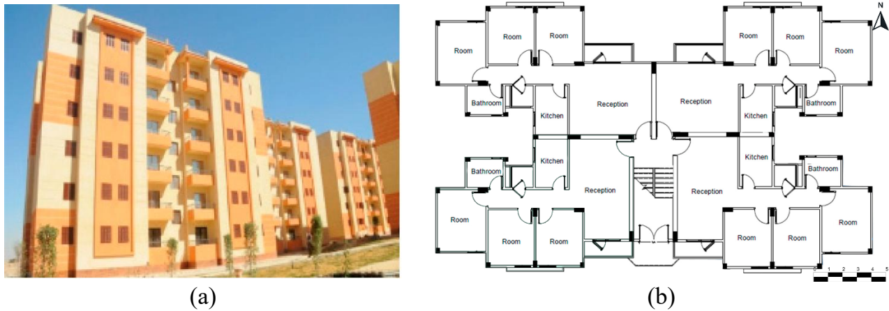
Fig. 2: The investigated residential building in New Aswan City: a) The exterior facades; b) The horizontal architectural drawing [43].
