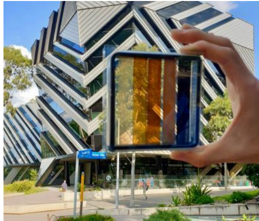
Fig. 6: Perovskite solar cell degrees of transparency [14].
